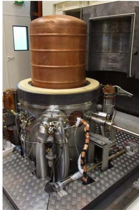
Fig. 16: Photo of the ^3\text{He} filled proportional counter installed at close proximity to the EDELWEISS-2 cryostat.
