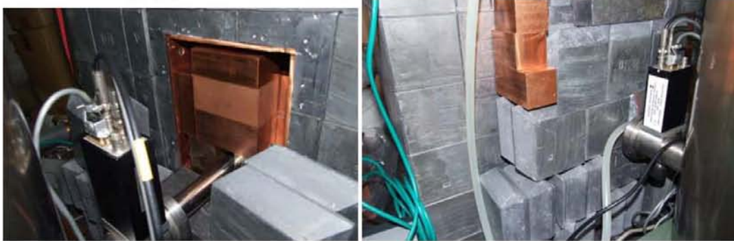
Fig. 24: View of the shield from side of cold finger, on the left – copper shield, on the right – lead shield with pipe of radon-free air supply.
