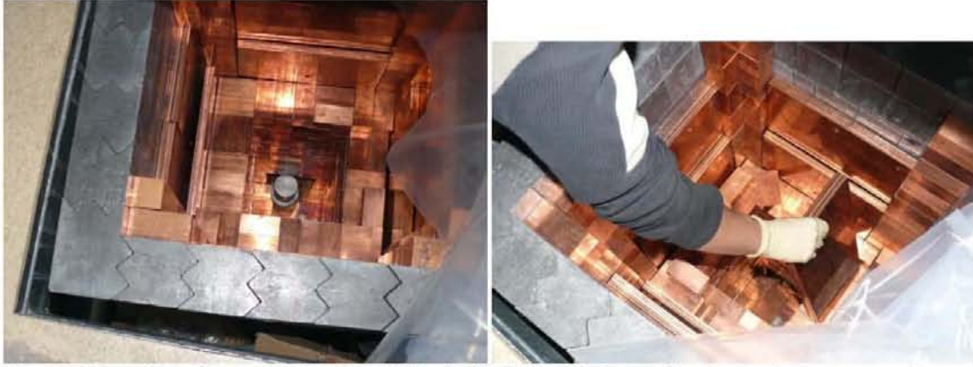
Fig. 23: View from the top of EDELWEISS1 shield (left) and photo of process of positioning of copper plates on the top (right).
