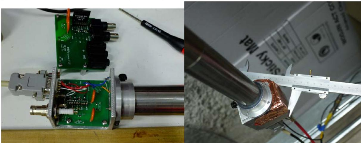
**Fig. 7.8:** Left: Old and new preamplifier part of thermal neutron detector. Right: the new preamplifier in its housing.
