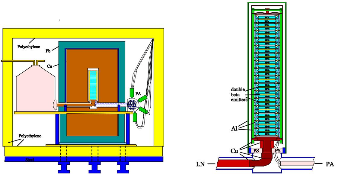
**Fig. 4.1:** Low background spectrometer TGV-2 (left part) and detector part with double beta emitters (right part).
