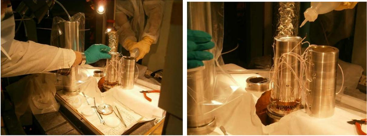
**Fig. 4.2:** *Disassembling of the TGV-2 detector system and installation of investigated samples.*
