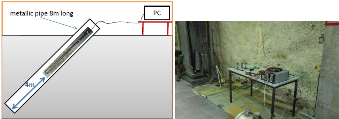
**Fig. 7.7:** Scheme (left) of the measurement of thermal neutrons deeply inside rocks and photo of the setup (right).
