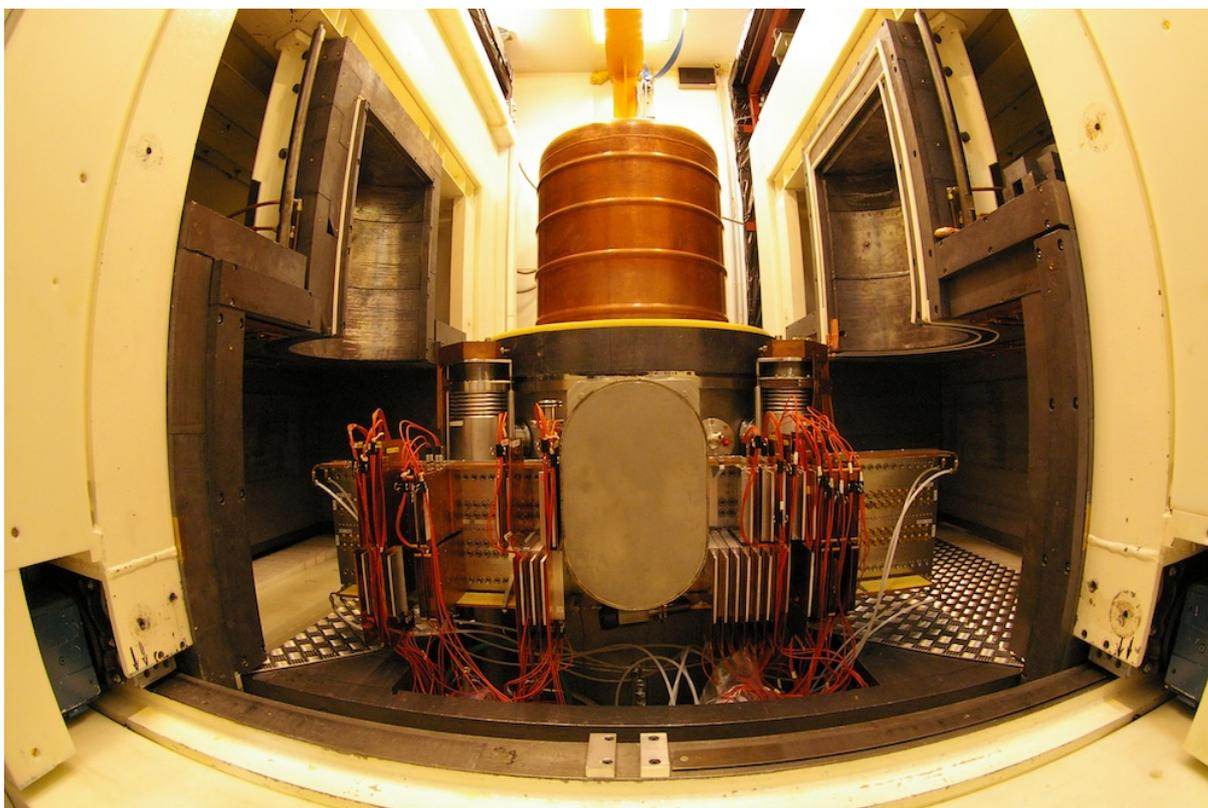
**Fig. 1.1:** *View of the assembled cryostat of the EDELWEISS (shield is open).*
