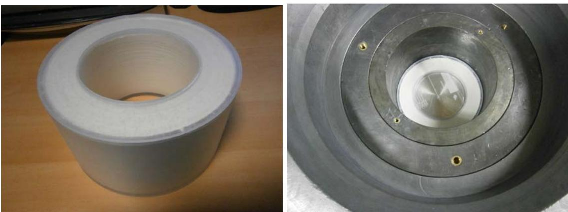
**Fig. 5.4.** A low-active sample on the base of  $\text{La}_2\text{O}_3$  in a bobbin (left part) and using the sample for the efficiency calibration of the detector (right part).
