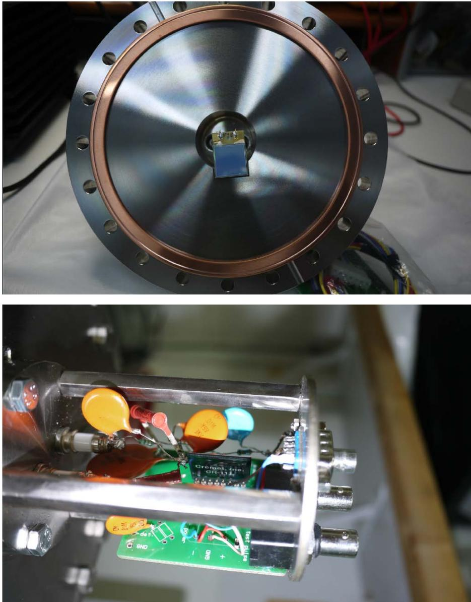
**Fig. 9.7:** *Top: new alpha detector installed into detector. Bottom: improved electronic part of the detector.*
