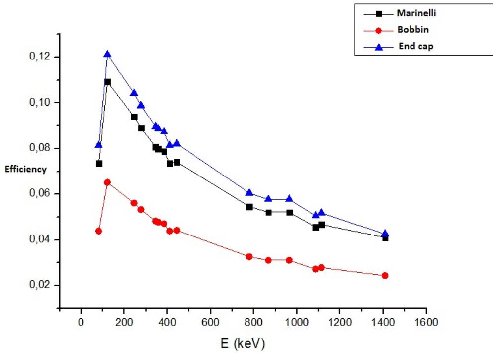
Fig.5.5. Efficiency curves for some “standard” geometries.
