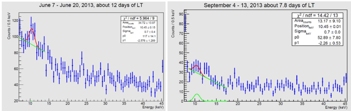
**Fig. 6.5:** Spectra received in June and September with ZZ-top detector inside of EDELWEISS-I shield. In beginning of June 2013 detector wrapping been changed from indium to archeological lead.
