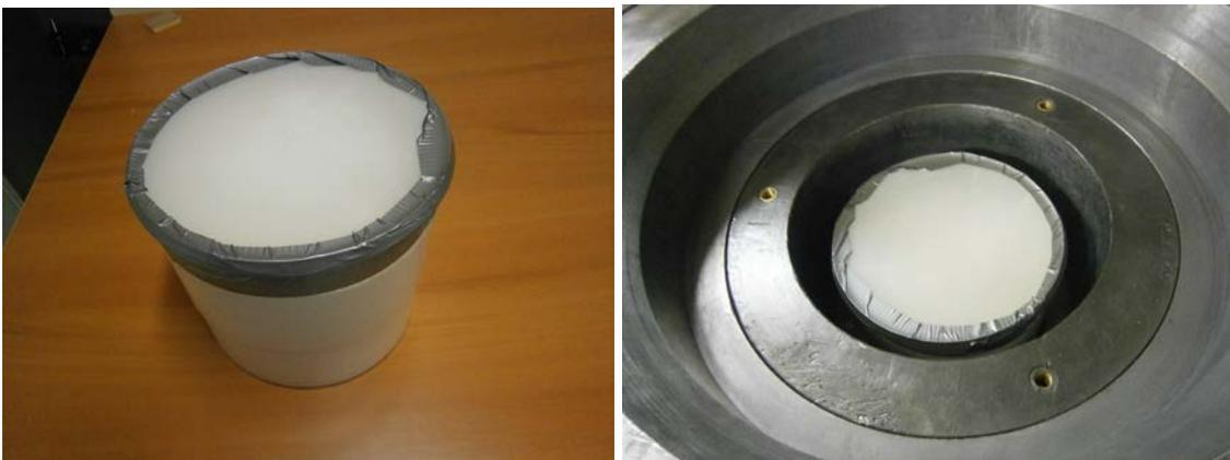
**Fig. 5.3.** A low-active sample on the base of  $\text{La}_2\text{O}_3$  in a big Marinelli beaker (left part) and using the sample for the efficiency calibration of the detector (right part).
