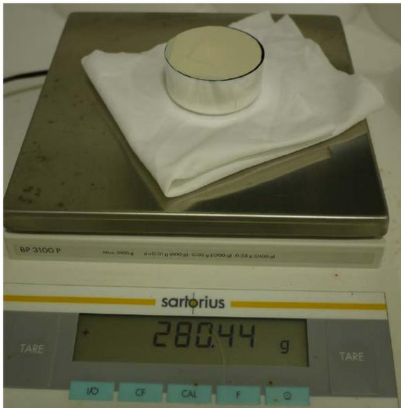
**Fig. 6.3:** *Weight measurement of ZZ-top HPGe crystal. The weight of Ge is 279.54 g.*
