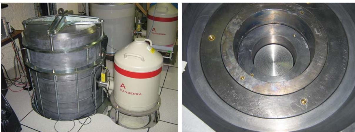
**Fig. 5.1:** Low background detector “Obelix” (left part) and inner part of a passive shielding (right part).
