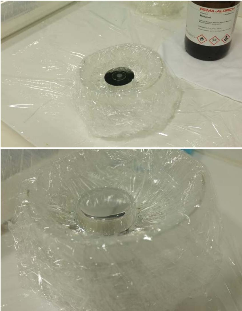
**Fig. 6.14:** *Cleaning of ZZ-top crystal by methanol.*
