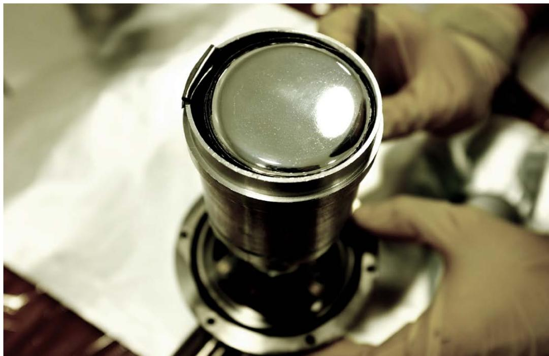
**Fig. 6.1:** View of the ZZ-top detector wrapped in archeological lead (inside of it holder). Work performed by E. Yakushev and S. Rozov in June 2013.
