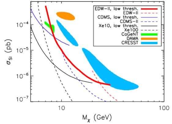
**Fig. 1.2:** Left: FID800 detector. Right: 90% C.L. Poisson limit on  $\sigma_{SI}$  as a function of WIMP mass derived from the analysis of the four EDELWEISS bolometers (bold red line).
