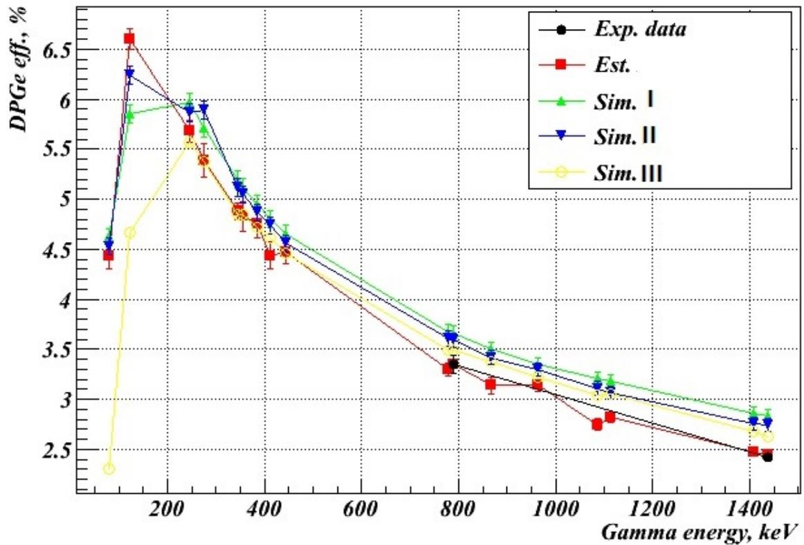
Fig.5.6. Efficiency curves of the HPGe spectrometer for measurement of Marinelli bobbin with metallic foil of  $^{100}\text{Mo}$  (experiment and MC simulations).
