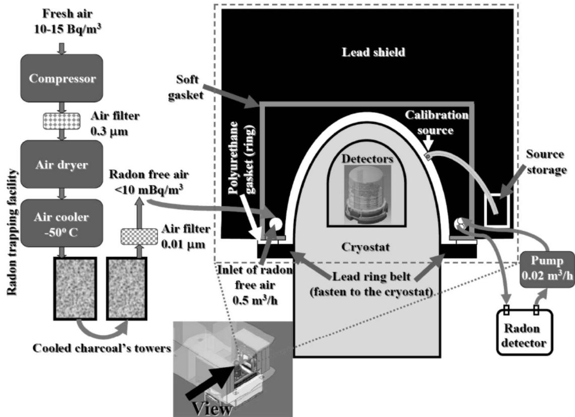
**Fig. 9.1:** Scheme of radon environment of EDELWEISS cryostat. Only upper part of the shield is shown.
