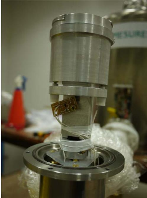
**Fig. 6.2:** *New first cascade of ZZ-top detector installed in March 2013.*
