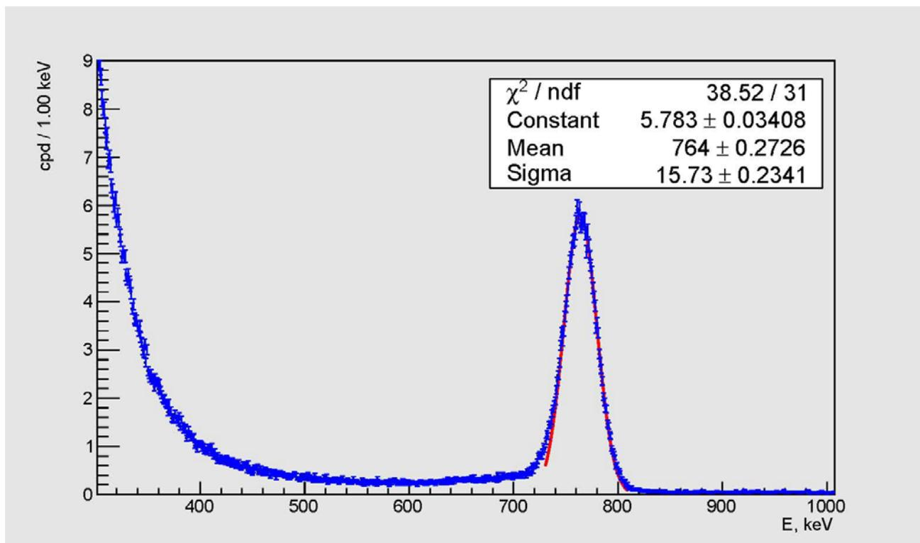
**Fig. 7.2:** *Experimental spectrum accumulated with 4 He-3 filled proportional counters in a polyethylene moderator (the detector of fast neutrons). The spectrum accumulated from September 2012 until August 2013.*
