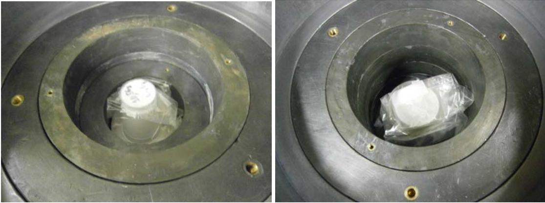
**Fig. 5.2:** Measurements of a small plastic box with powder of  $\text{La}_2\text{O}_3$  (left part) and a plastic box with a mix prepared on the base of  $\text{La}_2\text{O}_3$  (right part).
