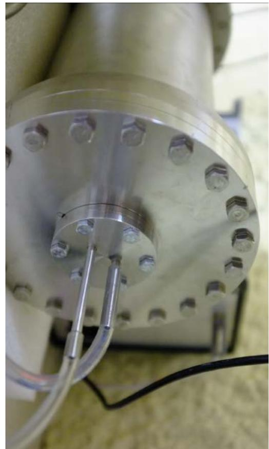
**Fig. 9.3:** Mobile high sensitive radon detection system.
